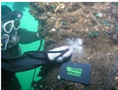
Photo-5.5.2 Plate thickness measurement using an ultrasonic thickness meter
