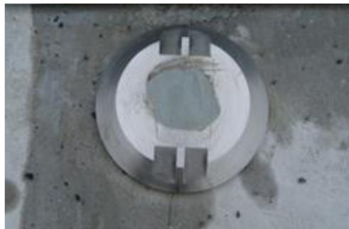
Photo-5.5.1 Potential measurement apparatus (terminal)
