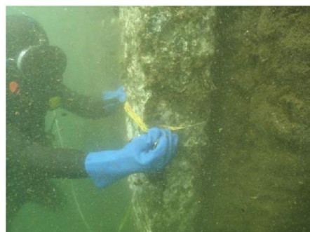
Photo-4.4.4 Image of measuring shape and dimensions of anode
