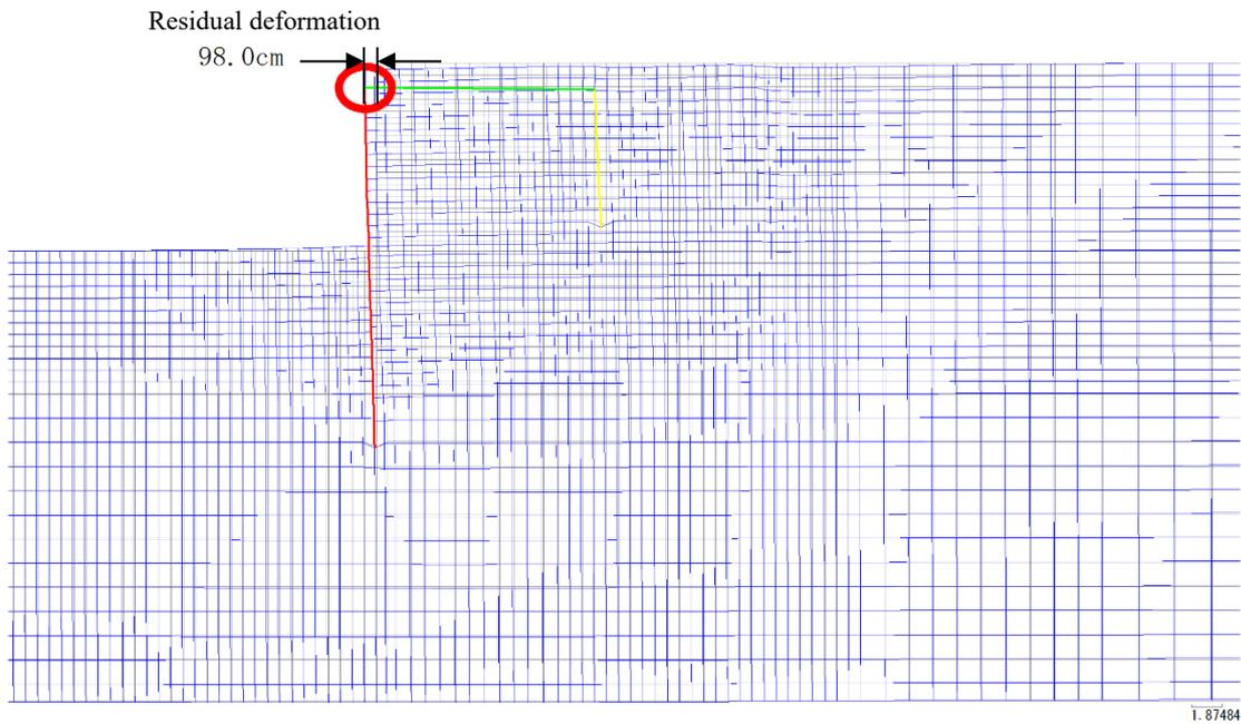
**Figure 5.3.23 Residual deformation diagram (Level 2 earthquake ground motion)**
