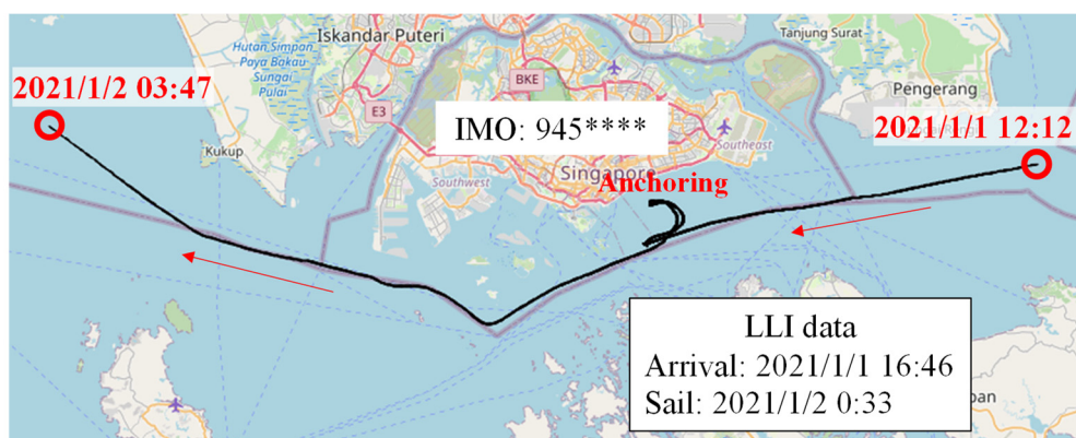
Figure 9 - Comparison LLI data with AIS data (Passing Ship)
