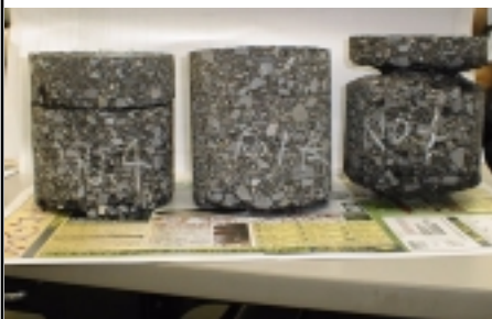
層間／骨材剥離
