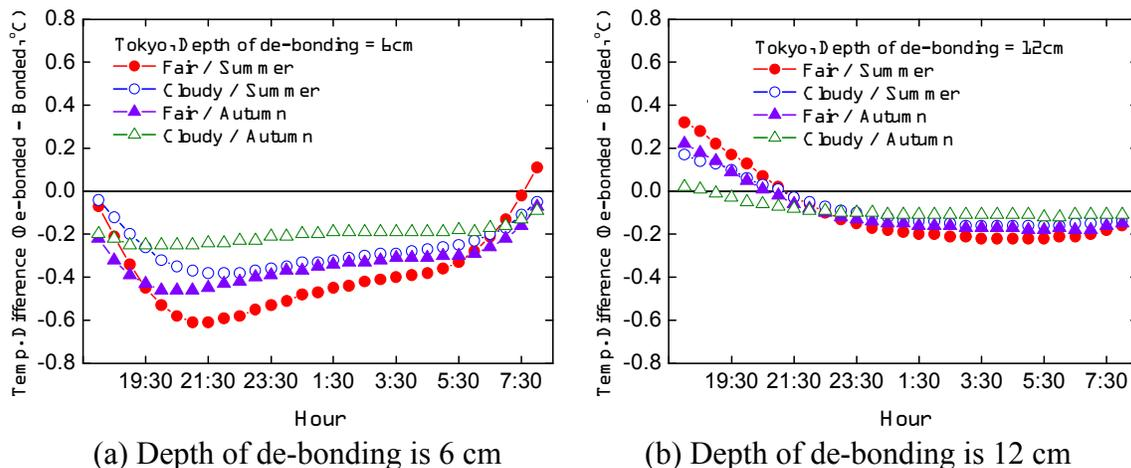
Figure 6 Variation of temperature difference on surface
