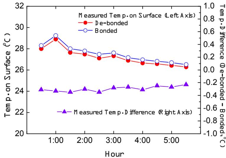
Figure 4 Variation of temperature and temperature difference on surface
