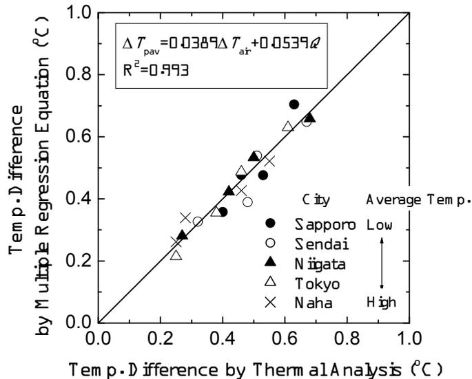
Figure 7 Result of multiple regression analysis (depth of de-bonding is 6 cm)
