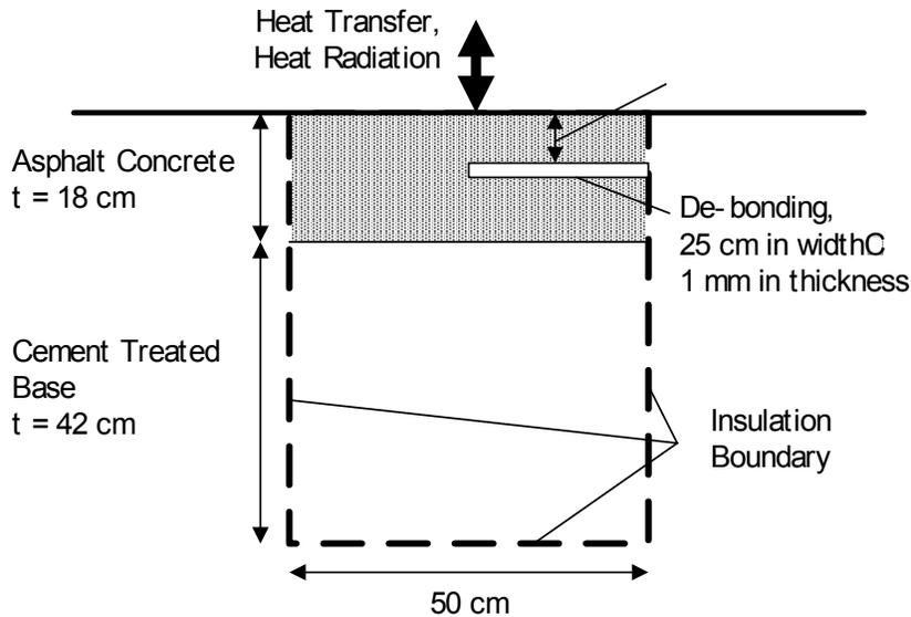
Figure 5 FEM model for thermal analysis
